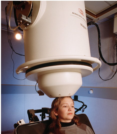
FIGURE 21 Magnetoencephalography. An array of SQUIDs in this neuromagnetometer detects regional changes in magnetic fields produced by electrical activity of the brain.
