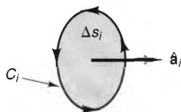
Figure 2-30 A surface \Delta s_i with unit normal \hat{\mathbf{a}}_i , bounded by the contour C_i .
