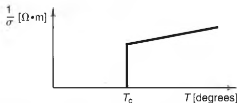
Figure 5-3 The resistivity of a superconductor as a function of temperature.
